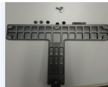
Step12. Remove six silicon rubbers
