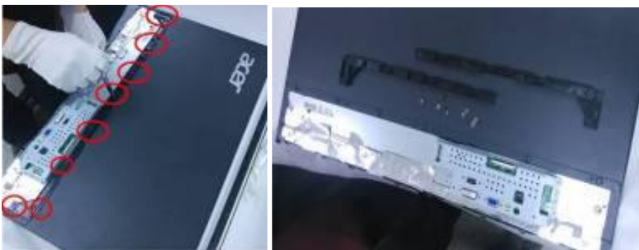
Step.7 Remove F/B and take out the LCM, then separate Key board from F/B and LVDS cable from LCM
