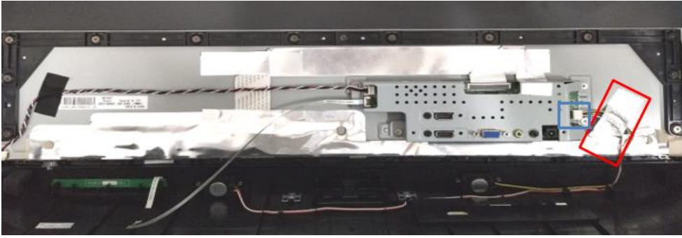
Step11. Assemble rear cover to LCM..
