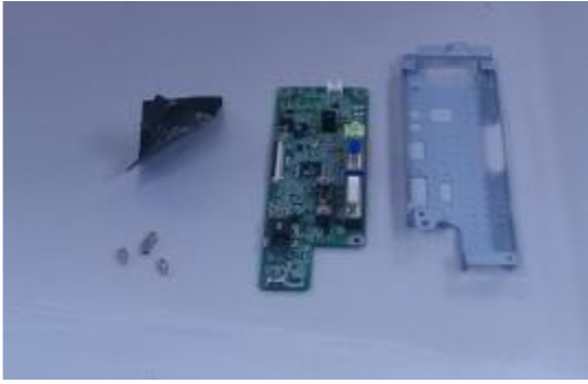
Step.10 Disassemble rear cover assembly
