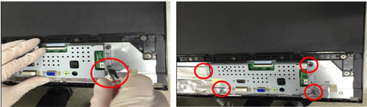
Step.6 Unscrew PCBA's screws and disassemble frame L&R.
